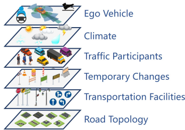
Fig. 2 Hierarchical scenario description. The communication status level is ignored from consideration as our focus is exclusively on the self-driving AD stack.
